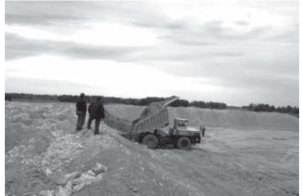
Stacking test heap utilizing "end dumping" method
