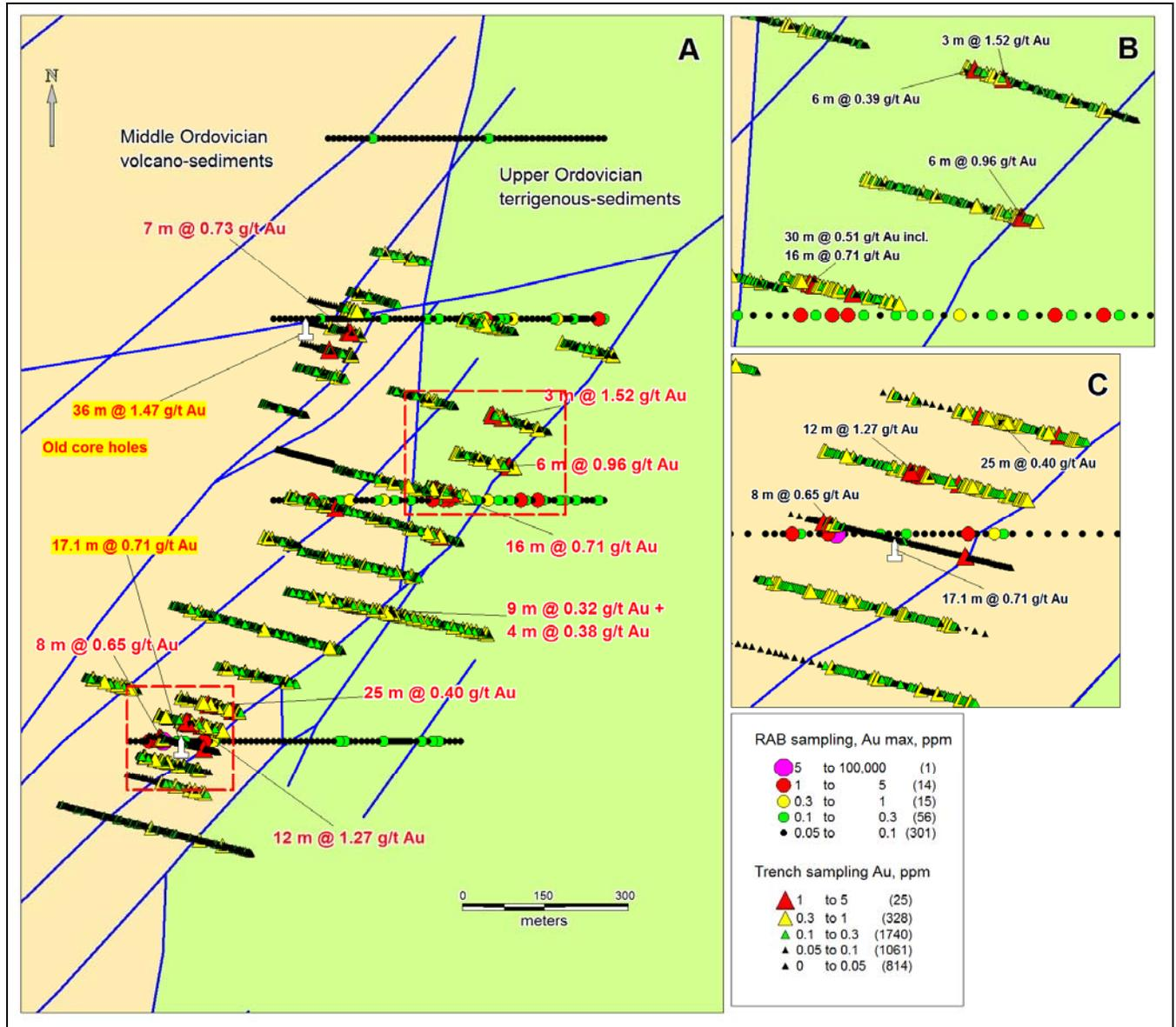
**Figure 4** - Kerbay trench and RAB sampling results (A) and zoom to the areas of planned drilling (B – northern and C – southern)
